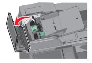
**4** Remove the pick roller assembly.
